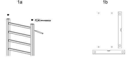
2. Using the drill and 8mm drill bit, drill into the marked positions then insert the wall plugs and tap flush to the finished wall surface.
